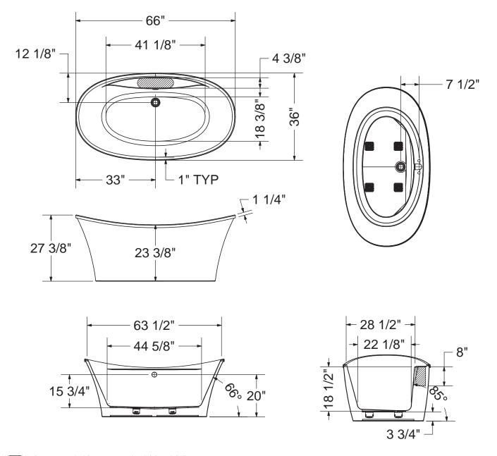
( Recommended faucet area of 15" (L) x 4" (W). Depth recommended for straight pipes 8".
